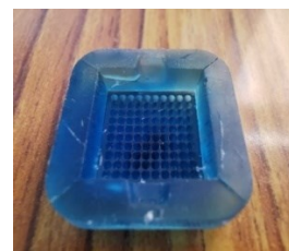
Figure 1 The fabricated microneedles mould
